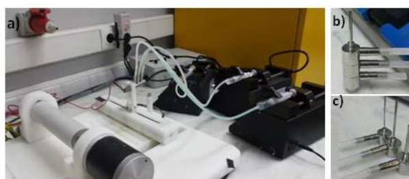
Fig. 1 (a) Co-axial Electrospinning setup (b) and (c) 3-ends nozzle
