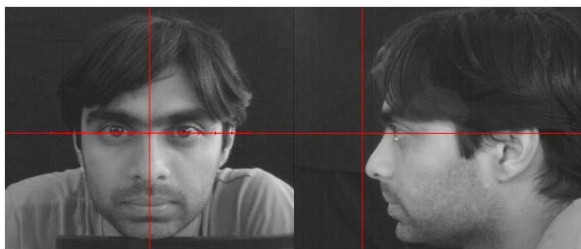
Fig. 1 Datum Lines for Initial Camera Set-up
