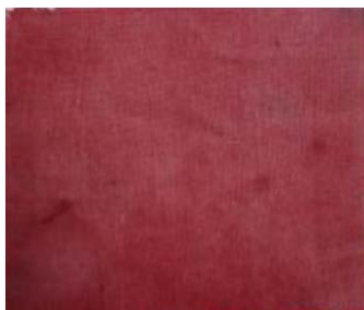
Fig. 5 Colour of a silk fabric sample dyed through simultaneous mordanting and dyeing procedures
