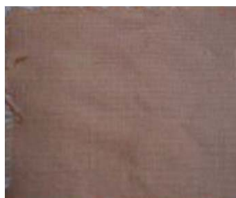
Fig. 6 Colour of a silk fabric sample dyed through post-mordanting and dyeing procedures
