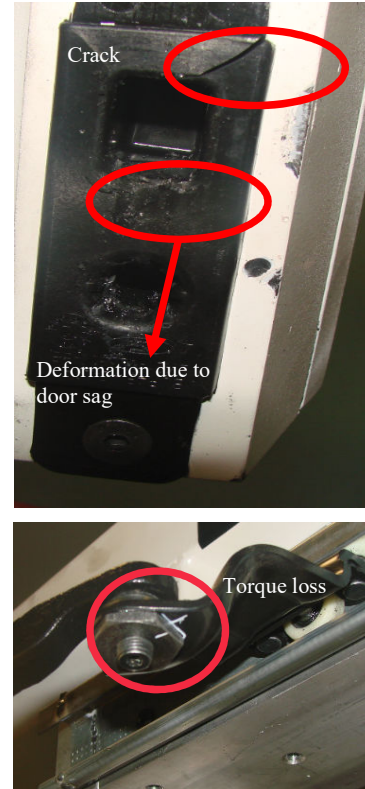
Fig. 13 Part fails from durability test [6]
