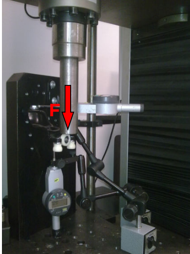
Fig. 12 Physical test set up for mechanism stiffness
