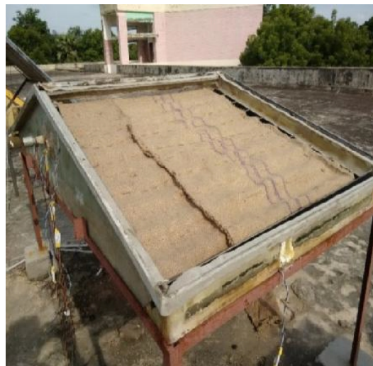
Fig. 2 Jute-Wick arrangement in MDSBMSS setup
