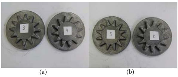
Fig. 8 Filling of the tooth shape: (a) after 5 blows; (b) after 9 blows; forgings 3, 5 are received with combined impact; forgings 4,6 - with simple impact
