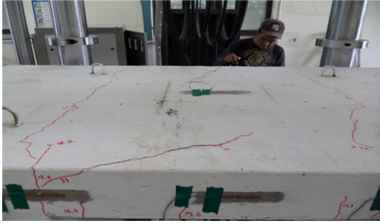
Fig. 11 Crack in ST Type
