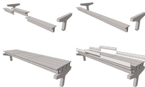
Fig. 1 Precast Modular Bridge System
