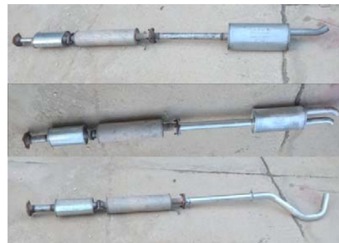
Fig. 2 Construction of the expansion chambers
