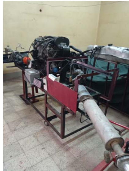
Fig. 1 Photo of the engine mounted on the test bench
