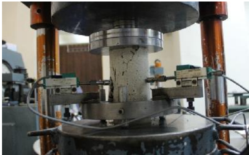
Fig. 3 Uniaxial compression test setup
