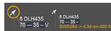
Fig. 14 Attention guidance elements for aircraft that have a short-term predicted conflict (orange circle around aircraft in automation level 0, orange alpha-numeric values in automation level 1)
