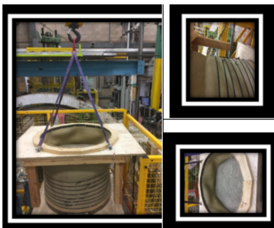
Fig. 2 Soil Container Fixed on Shaking Table at Salford University
