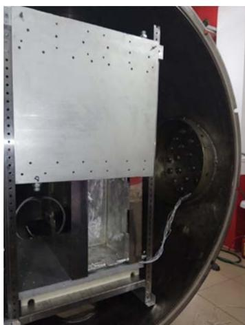
Fig. 22 Mounting mirror steel box inside the MVC
