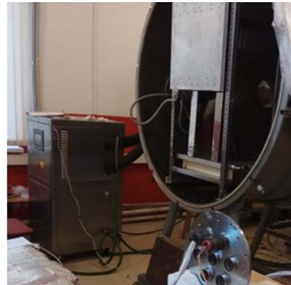
Fig. 14 Cooling system for the MVC
