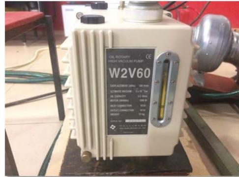
Fig. 18 Rotary high vacuum pumps Model W2V60
