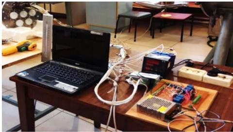
Fig. 10 Computer and data acquisition
