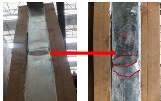
(b) Local buckling of W-2 CFS
