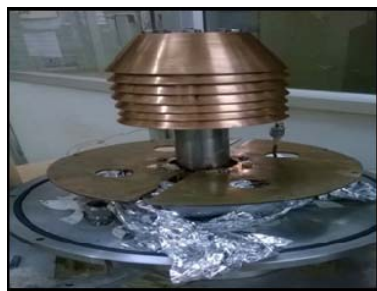
Fig. 4 Bare cryopanel mounted on the cryocooler
