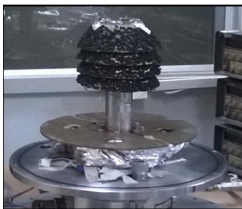
Fig. 7 Cryopanel with Activated Carbon
