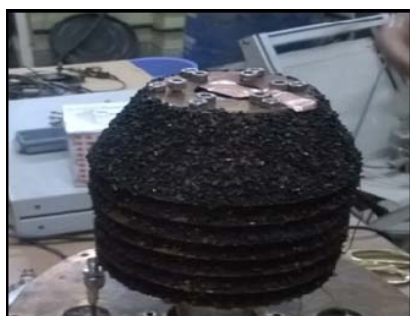
Fig. 9 Cryopanelcoated with smaller Activated Carbon
