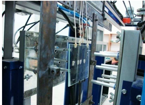
Fig. 3 Cooling nozzle arrays in staggered arrangement
