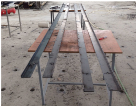
Fig. 3 L shape steel made-up sections used as longitudinal reinforcement in boundary regions of the CSW test specimen
