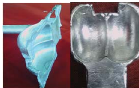
Fig. 9 The defect-free Pelton bucket cast
