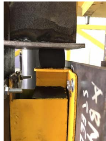
Fig. 4 Deformation of the damper
