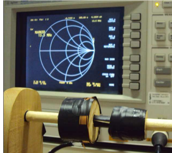
Fig. 7 Mutual inductance measurement
