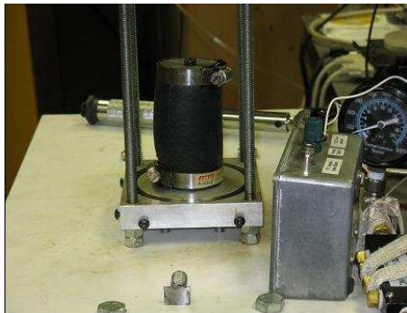
Fig. 4 Rubber bladder used to contain the propellant
