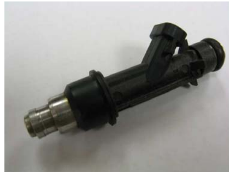
Fig. 1 Photograph of the type of fuel injector used to meter the propellant (linear dimension is 8 cm).
