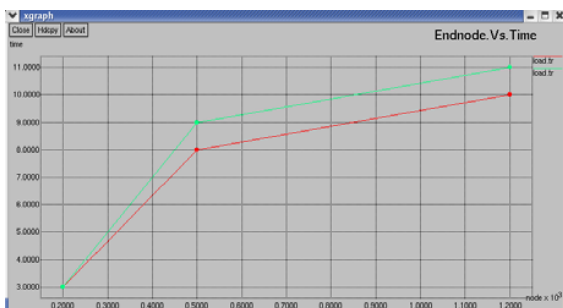
Fig. 6 Dijkstra's and QoS based algorithm under various loads
