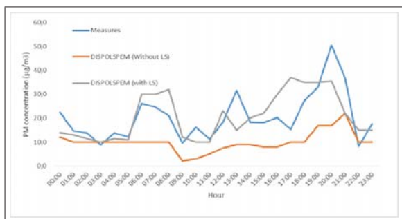
Fig. 14 Time evolution of measured and simulated concentrations of PM with and without taking into account the road traffic emissions (line sources) in \mu gm^{-3}
