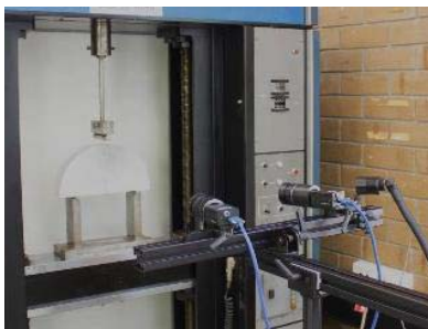
Fig. 4 Vic-3D (Correlated Solutions, Inc.) set up for the measurement of out-of-plane surface displacement
