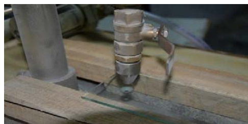
Fig. 2 Hole formation on glass sheet
