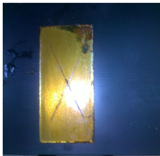
Fig. 6 Salt spray resistance of PU5 after 950 hours
