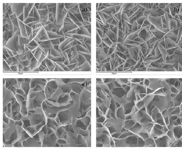
Fig. 5 SEM micrographs of BSA incorporated calcium phosphate coatings produced by rapid biomimetic co-precipitation technique. The concentrations of protein solution used were: a)  $0 \mu\text{g ml}^{-1}$ ; b)  $1 \mu\text{g ml}^{-1}$ ; c)  $10 \mu\text{g ml}^{-1}$ ; d)  $100 \mu\text{g ml}^{-1}$  (Magnification  $\times 5,000$ , Scale bar =  $10 \mu\text{m}$ )
