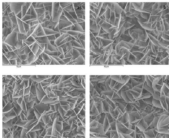
Fig. 4 SEM micrographs of BSA incorporated calcium phosphate coatings produced by direct adsorption technique. The concentrations of protein solution used were: a)  $0 \mu\text{g ml}^{-1}$ ; b)  $1 \mu\text{g ml}^{-1}$ ; c)  $10 \mu\text{g ml}^{-1}$ ; d)  $100 \mu\text{g ml}^{-1}$  (Magnification  $\times 5,000$ , Scale bar =  $10 \mu\text{m}$ )
