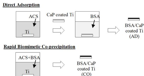
Fig. 1 Process diagram showing protein incorporation in the calcium phosphate coating used in this study
