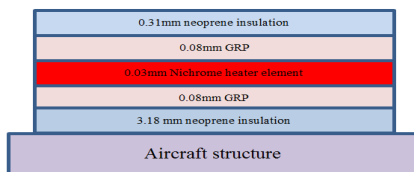
Fig. 3 Layout of heater mat model used for the calculation
