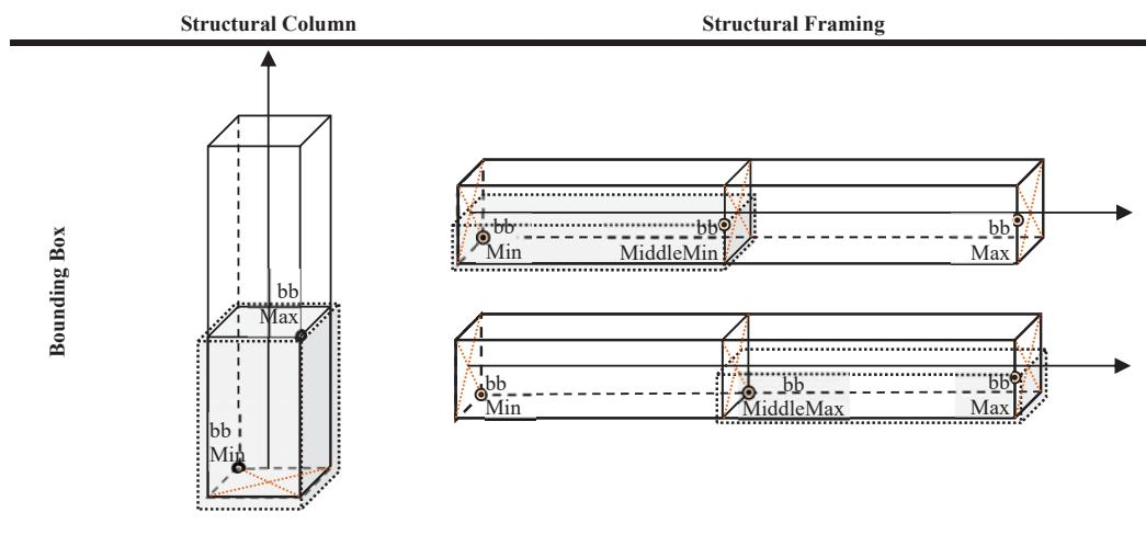
Fig. 9 Structural Column and Structural Framing Bounding Boxes
