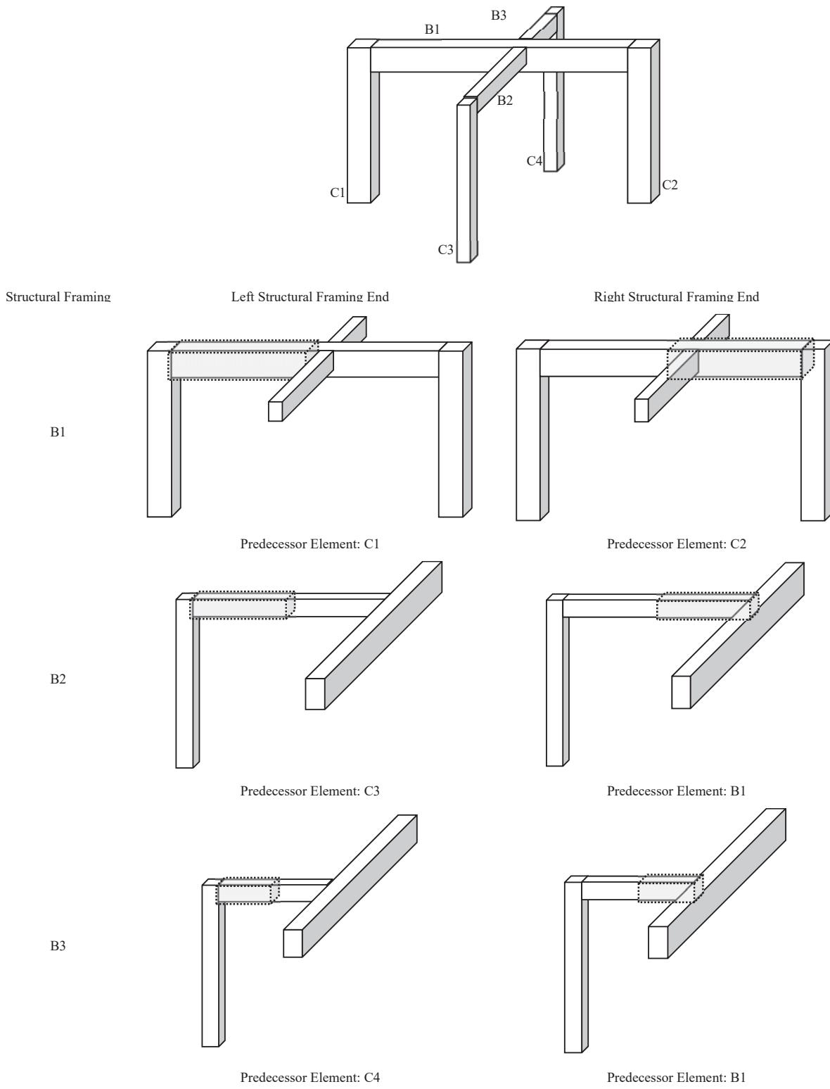
Fig. 11 Structural Framing Dependency – 2 Intersecting Frames
