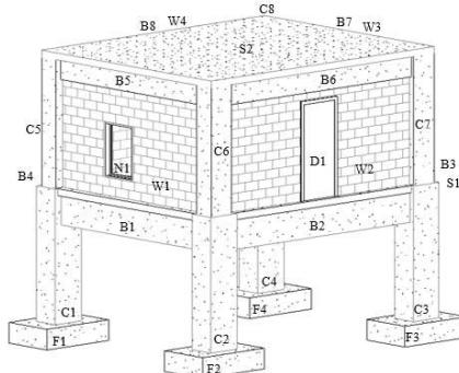
Fig. 7 Example No. 2 and its Elemental Graph (4 foundations, 8 columns, 8 beams, 2 slabs, 4 walls, door, and window)
