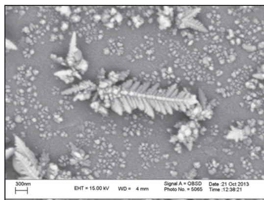
Fig. 2 SEM image of silver nanostructures that prepared at a deposition time 120 s and deposition potential -0.1 V
