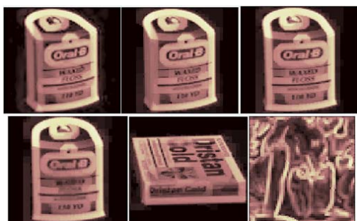
Fig. 9 Morphological Gradient with EZW Compressed Sequence images
