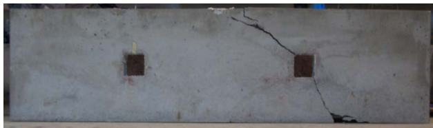
Fig. 11 Crack pattern for beam S05-80-3 [12]
