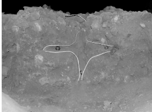
Fig. 5 Lateral and vertical separation of seed and fertilizer in the slot created by modified double disks opener
