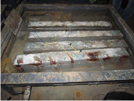
Fig. 3 Accelerated Corrosion Process for Unstressed Condition
