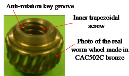
Fig. 9 Design process of the worm wheel, showing a photo of the real wheel made in CAC502C bronze
