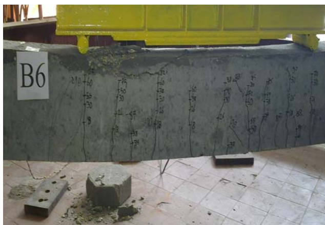
Fig. 7 Typical flexure failure for beam specimens
