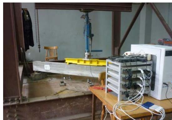
Fig. 4 Splice beam prior to testing
