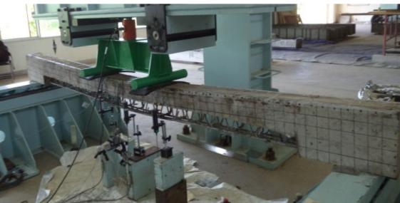
Fig. 6 Specimen Under Loading
