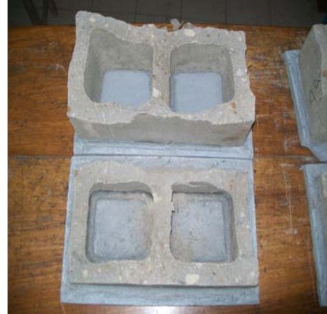
Fig. 3 Fracture shape of sandcrete block specimens
