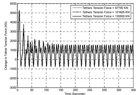
Fig. 17 Change in tether tension force of square TLP for Wave Height = 10 m and wave period = 15 sec
