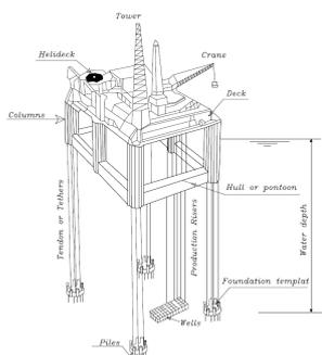
Fig. 2 Tension leg platform scheme
