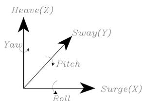
Fig. 1 Six degree of freedom of offshore structure
