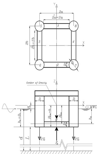
Fig. 3 The Square TLP (plan and elevation)
