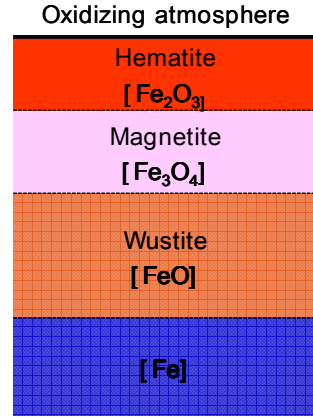
Fig. 1 Schematic representation of the typical scale layers on the slab surface exposed to oxidizing furnace environments
