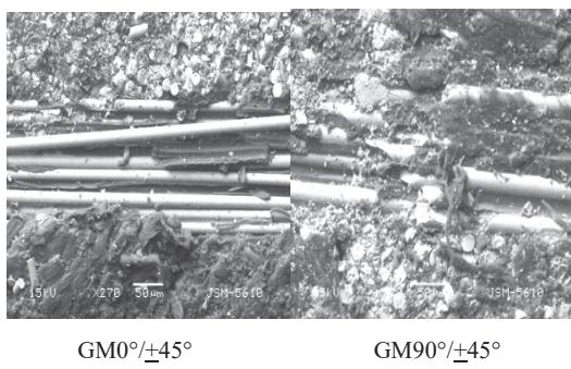
(b) Preform Structure in Laminate
