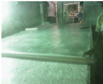
Fig. 2 Hand Laying Process
