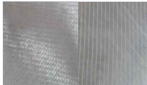
(a) GM  $0^\circ, \pm 45^\circ$  CDB (Tricot) (b) GM  $90^\circ, \pm 45^\circ$  DDB(Pillar)
