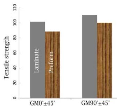
Fig. 8 Tensile Strength of Glass Preforms and Laminate
