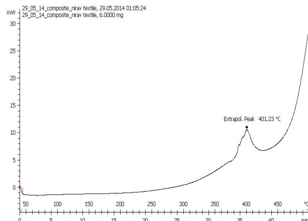
Fig. 6 DSC Analysis of Glass Laminate ( $GM0^\circ/\pm45^\circ$ )
