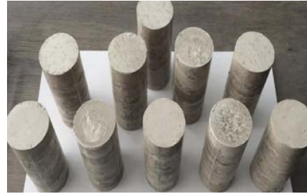
Fig. 3 prepared specimens for UCS test
