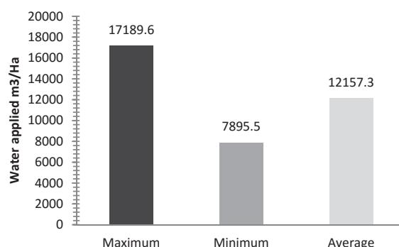
Fig. 4 Water applied m<sup>3</sup>/Ha for farms with surface irrigation
