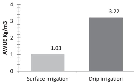
Fig. 7 Effect of the irrigation system on the AWUE
