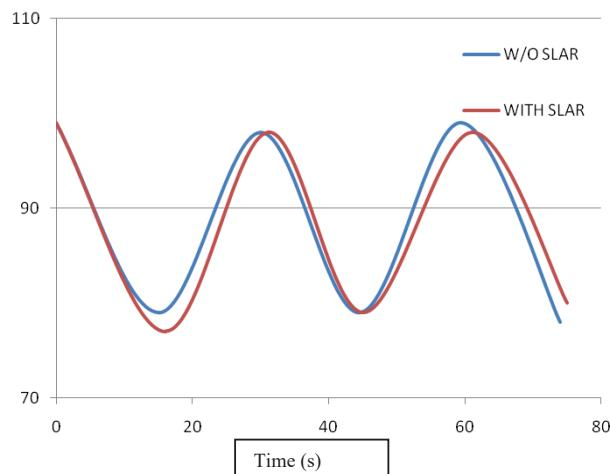
Fig. 2 Comparative plot for Phugoid motion in landing configuration
