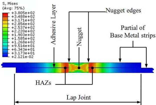
Fig. 9 Contour residual stresses for FE weld-bonded model
