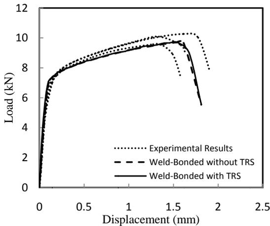
Fig. 10 Load-displacement curves for FE and experimental results of weld-bonded joints.
