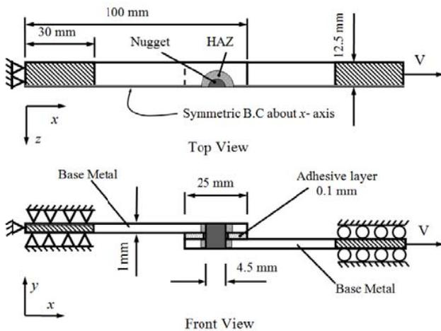
Fig. 5 Weld-Bonded Models
