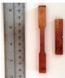
Fig. 4 Tensile and impact test specimens
