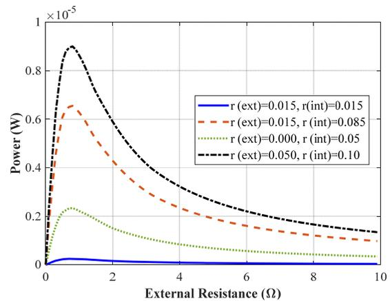
Fig. 4 Highest output power under different damping coefficient
