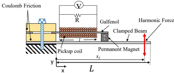
Fig. 1 Schematic view of Galfenol harvester
