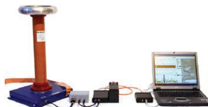
Fig. 3 MPD540 advanced PD measuring system with coupling capacitor
