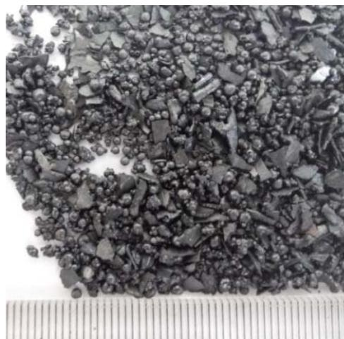
Fig. 2 Particle morphology of granulated slag
