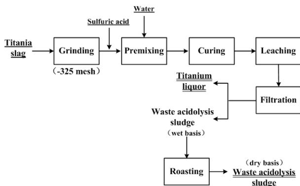
Fig. 3 Flow chart of acidolysis process of cooled slag
