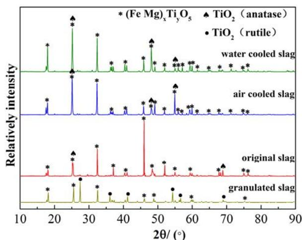
Fig. 4 XRD Patterns of cooled slag and the original slag
