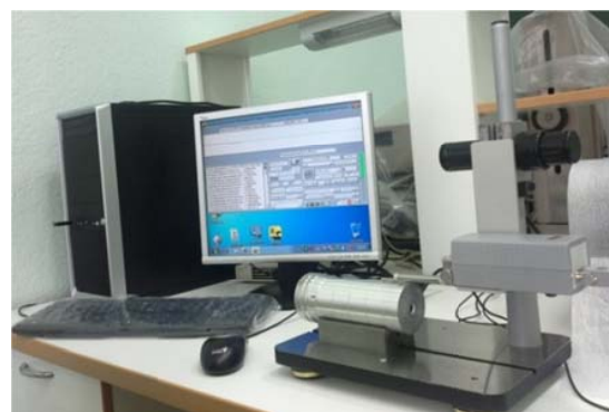
Fig. 3 Measuring surface roughness using profilemeter model 130
