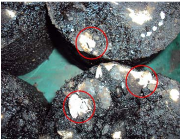
Fig. 4 Broken aggregates during compaction
